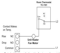
Typical unit heater application wiring for strap-on thermostat TC-2974 Unit heater fan runs only when heating supply media is above the setpoint of TC-2974
